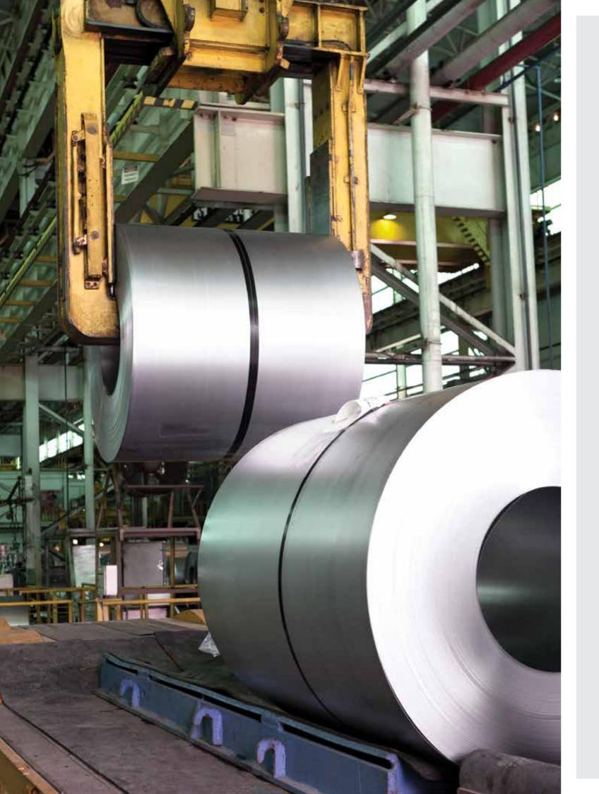
Cold rolled steel is generated by cold reduction applied to hot rolled product, followed by subsequent annealing (heat treatment).
